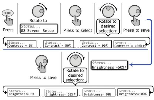
Figure 3-13, SETUP: 08 Screen Setup Selections
