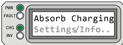
**Absorb Charging** appears on LCD; PWR (green) is on solid and CHG (green) LED is typically on solid, but may blink slowly. FAULT (red) LED is off. INV (green) LED could be on or off.
