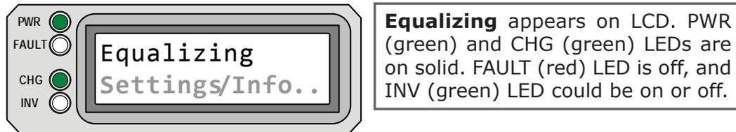
Figure 5-11, Equalizing Mode
