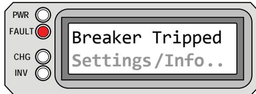
**Breaker Tripped** appears on the LCD. The FAULT (red) LED is on. The PWR (green), CHG (green), and INV (green) LEDs are off.
