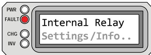
**Internal Relay** appears on the LCD. The FAULT (red) LED is on. The PWR (green), CHG (green), and INV (green) LEDs are off.
