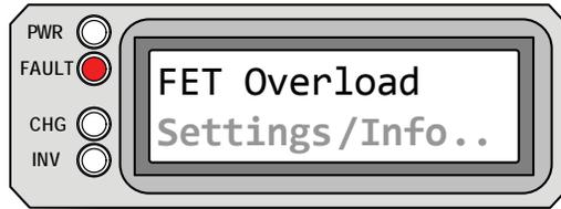
**FET Overload** appears on the LCD. The FAULT (red) LED is on. The PWR (green), CHG (green), and INV (green) LEDs are off.
