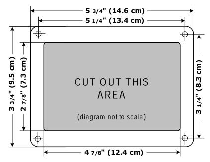
Figure 2-1, Remote Cut-out Dimensions
