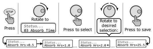
Figure 3-8, SETUP: 03 Absorb Time Selections
