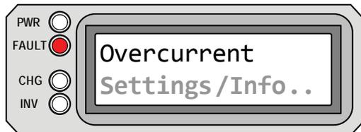
**Overcurrent** appears on the LCD and the FAULT (red) LED is on. The PWR (green), CHG (green) and INV (green) LEDs are off.
