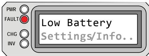
**Low Battery** appears on the LCD. The FAULT (red) LED is on. The PWR (green), CHG (green), and INV (green) LEDs are off.
