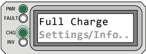
**Full Charge** appears on LCD. PWR (green) LED is on solid, and CHG (green) LED blinks slowly. FAULT (red) LED is off, and INV (green) LED could be on or off.
