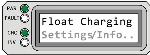
**Float Charging** appears on LCD. PWR (green) LED is on solid, and CHG (green) LED is typically on solid, but may blink slowly. FAULT (red) LED is off, and INV (green) LED could be on or off.
