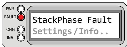
**StackPhase Fault** appears on the LCD. The FAULT (red) LED is on. The PWR (green), CHG (green), and INV (green) LEDs are off.
