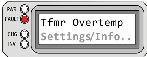
**Tfmr Overtemp** appears on the LCD. The FAULT (red) LED is on. The PWR (green), CHG (green), and INV (green) LEDs are off.
