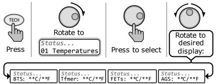
Figure 3-14, TECH: 01 Temperatures Display
