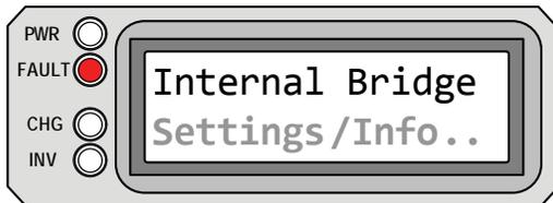
**Internal Bridge** appears on the LCD. The FAULT (red) LED is on. The PWR (green), CHG (green), and INV (green) LEDs are off.
