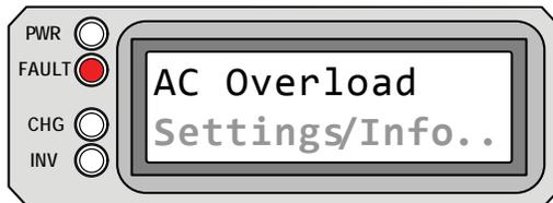
**AC Overload** appears on the LCD. The FAULT (red) LED is on. The PWR (green), CHG (green), and INV (green) LEDs are off.
