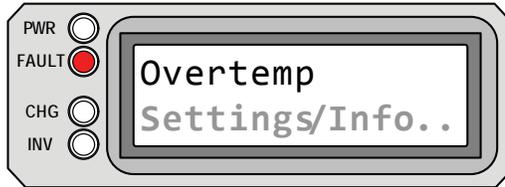
**Overtemp** appears on the LCD. The FAULT (red) LED is on. The PWR (green), CHG (green), and INV (green) LEDs are off.
