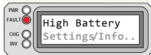
**High Battery** appears on the LCD. The FAULT (red) LED is on. The PWR (green), CHG (green), and INV (green) LEDs are off.
