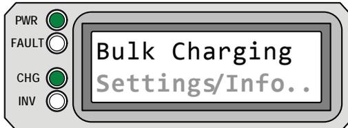
**Bulk Charging** appears on LCD. PWR (green) is on solid, and CHG (green) LED is typically on solid, but may blink slowly. FAULT (red) LED is off. INV (green) LED could be on or off.
