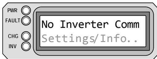
**No Inverter Comm** appears on the LCD. The FAULT (red), PWR (green), CHG (green), and INV (green) LEDs are normally off.
