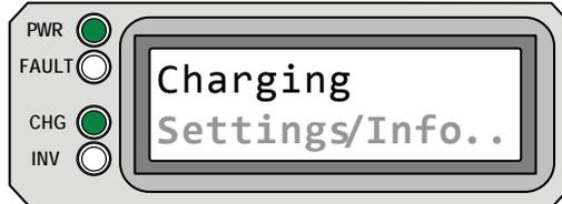
**Charging** appears on LCD. PWR (green) and CHG (green) LEDs are on solid. FAULT (red) LED is off, and INV (green) LED could be on or off.
