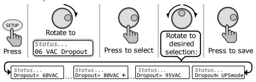
Figure 3-11, SETUP: 06 VAC Dropout Selections
