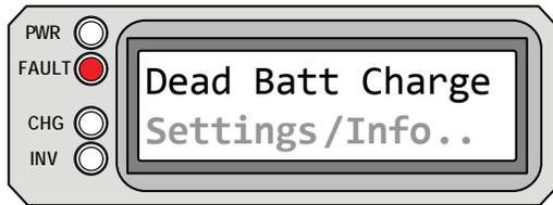
**Dead Battery Charge** appears on the LCD. The FAULT (red) LED is on. The PWR (green), CHG (green), and INV (green) LEDs are off.
