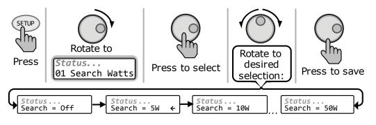
Figure 3-6, SETUP: 01 Search Watts Selections
