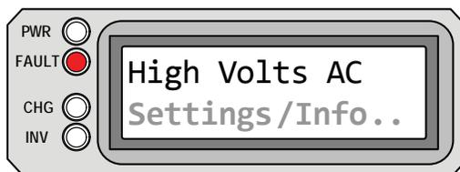
**High Volts AC** appears on the LCD. The FAULT (red) LED is on. The PWR (green), CHG (green), and INV (green) LEDs are off.
