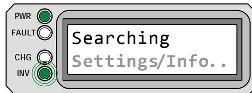
**Searching** appears on the LCD. The PWR (green) LED is on solid, and the INV (green) LED slowly flashes. The FAULT (red) and CHG (green) LEDs are off.
