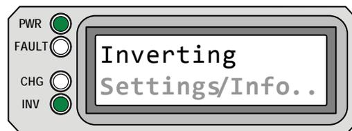
**Inverting** appears on the LCD. The PWR (green) and INV (green) LEDs are on solid. The FAULT (red) and CHG (green) LEDs are off.
