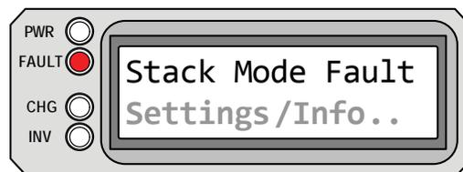
**Stack Mode Fault** appears on the LCD. The FAULT (red) LED is on. The PWR (green), CHG (green), and INV (green) LEDs are off.
