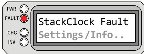
**StackClock Fault** appears on the LCD. The FAULT (red) LED is on. The PWR (green), CHG (green), and INV (green) LEDs are off.
