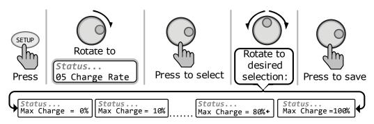
Figure 3-10, SETUP: 05 Charge Rate Selections
