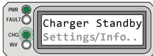
**Charger Standby** appears on LCD. PWR (green) LED is on solid and CHG (green) LED slowly blinks. FAULT (red) LED is off, and INV (green) LED could be on or off.
