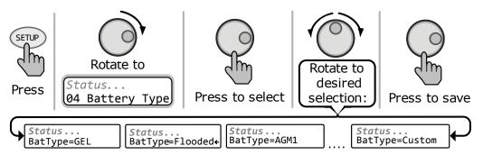
Figure 3-9, SETUP: 04 Battery Type Selections
