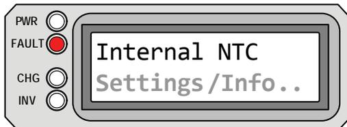
**Internal NTC** appears on the LCD. The FAULT (red) LED is on. The PWR (green), CHG (green), and INV (green) LEDs are off.
